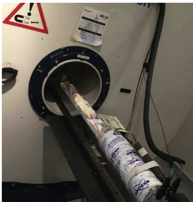
Figure 2 Anesthetized animals were monitored for temperature and respiratory frequency during MRI analysis. High resolution T2-weighted fast spin-echo sagittal images were acquired of the injured and contralateral patellar tendons.
